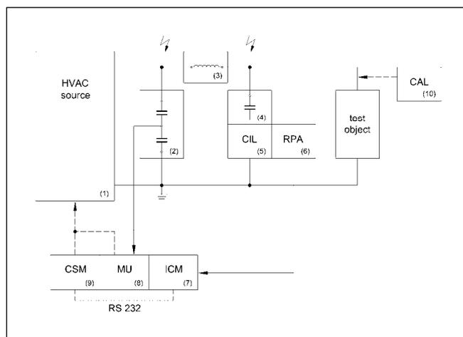
Fig. 1: PD measuring circuit according to IEC 60270 (explanations in the text)
