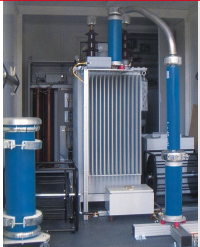
Fig. 2 Portable HVAC resonant test system type WR container variation
